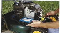
■ Replace the mower's air filter per manufacturer's recommendations—it is held in place with a spring clamp or screws.
