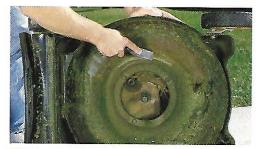
In the blade housing should be scraped clean after each use. Also scrape off dried grass on the clipping bags and chutes.
