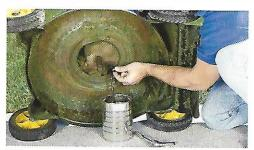
At least once a year, remove the blade for sharpening, and replace the engine oil to get the most out of the engine's life.
