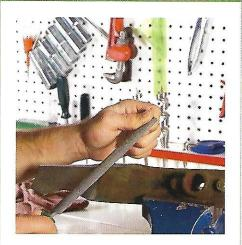
To sharpen rotary mower blades with a file, first disconnect the engine's spark plug before removing the blade. While sharpening, preserve the original angle of the sharpened edge as you stroke the file across it. File in one direction only-away from you. After you've sharpened each blade end, check the blade balance by slipping the center hole over a nail protruding from the wall. If the blade dips to one side or another, file away some more metal from that end.
