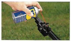
**5 Controls** should be cleaned out and coated with a lubricating oil at the beginning of each season.
