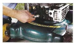
☑ Change the spark plugs regularly you'll need a socket wrench and a deepwell socket to loosen the plug.
