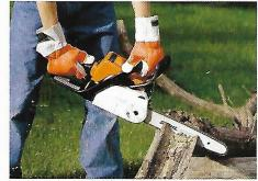
Chain saws with bars over 36 in. long are expensive, and heavy—most people can get by with a 16- to 20-in. bar.
