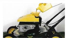
**6** Check the oil after each use, and top it off whenever necessary. It will keep the engine running smoothly and extend its life.
