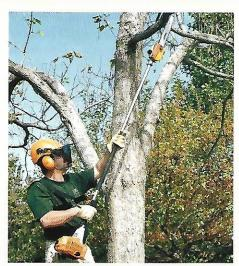
For trimming high branches, a power pruner is much easier than a pole saw.
